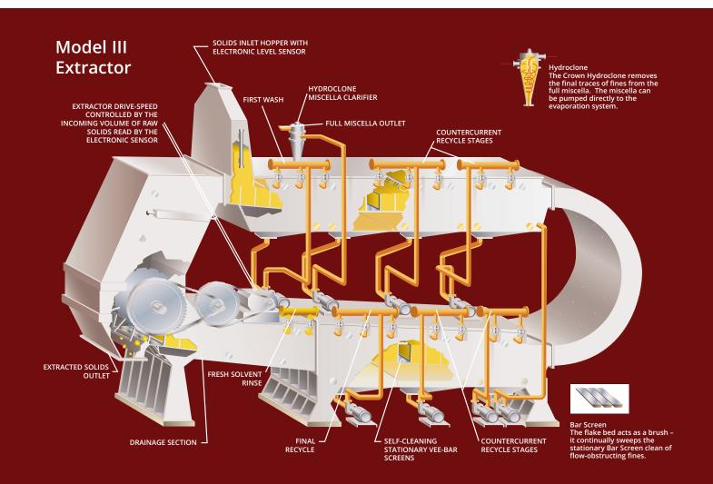
From the fresh solvent wash section, the miscella travels from stage to stage, counter-current along the bottom section of the extractor. At the end of the bottom section, an automatic level controller pumps or lifts the miscella to the top section of the extractor. From here the process is repeated until the final or full miscella is removed from the last washing stage on the top section.
