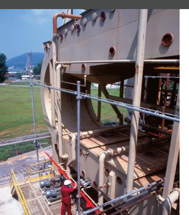
Crown's Model III Continuous Loop Shallow Bed Extractor offers the benefits of low power requirements, excellent component life, ease of operation and the capability of high operating capacities. The Crown design is the most efficient of several methods of extracting vegetable oils from oil-bearing seeds. This design maximizes extraction efficiency while at the same time minimizing steam consumption.
