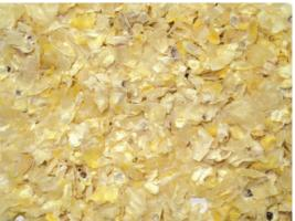
CPM Crown's Fractionation System separates corn into three components: starch, germ and bran. Separating the non-fermentable products such as germ and bran from the starch increases an ethanol plant's efficiency and throughput per bushel and is the first step to creating value-added co-products.
